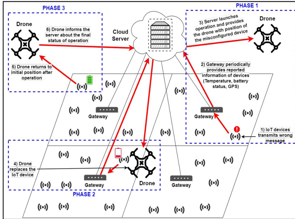
Fig. 1. Centralized architecture for managing drone operations
