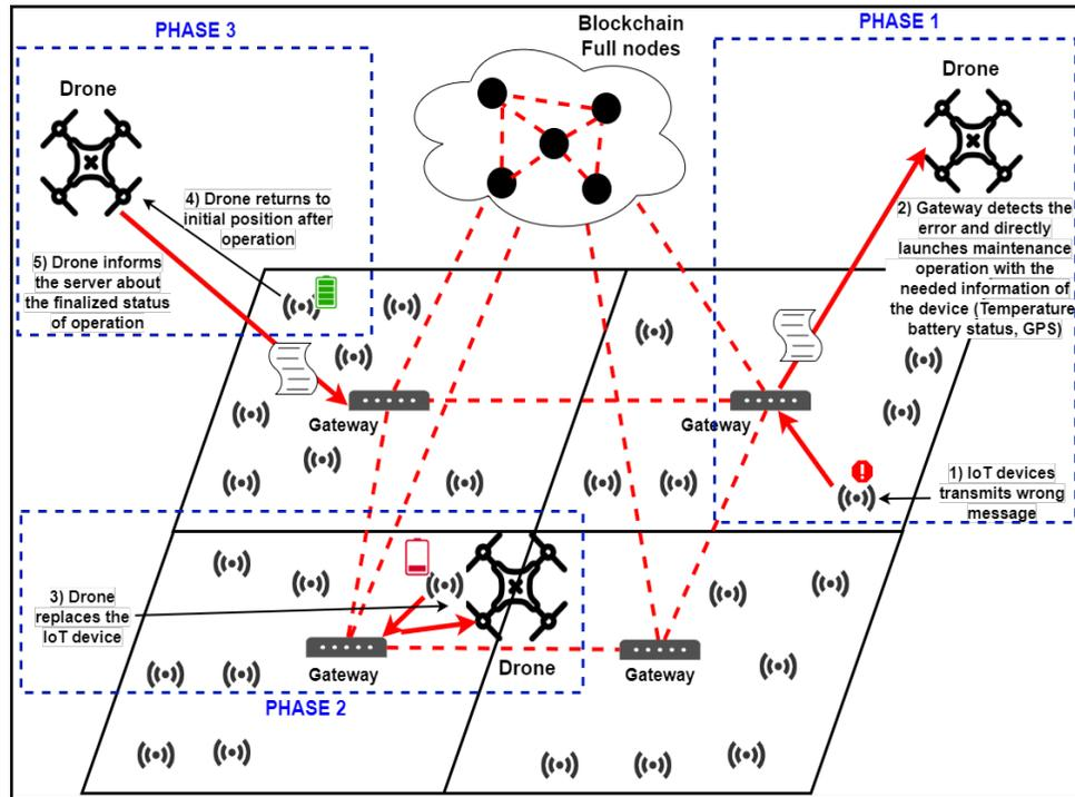
Fig. 2. Decentralized Blockchain-based architecture for managing drone operations
