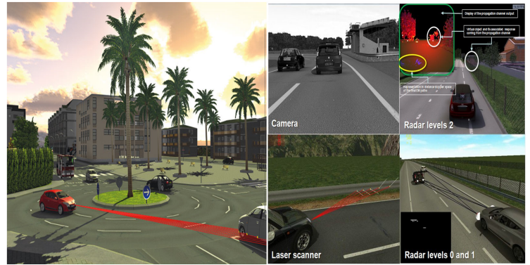
Fig. 4: Example of Pro-SiVIC environment where the ego-vehicle is equipped by multiple sensors.
