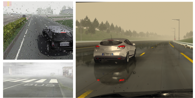
Fig. 5: Example of Pro-SiVIC weather conditions simulation (rain drops, inhomogeneous fog, and wet road surface).
