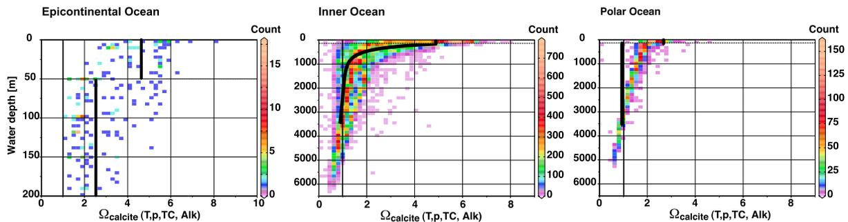
**Fig. 9.** Simulated steady state depth profiles of saturation state ( $\Omega_{\text{calcite}}$ ) in the epicontinental, inner and polar ocean (black line). Simulation results are compared to calcite saturation calculated based on WOCE Hydrographic Program (\*hy1.csv files from WHPO web-site as of 27 May 2002) observations using the in-situ temperature, pressure,  $T_C$  and  $T_A$  (Fig. 7). The colour code indicates the number of times a concentration is reported for a given water depth.
