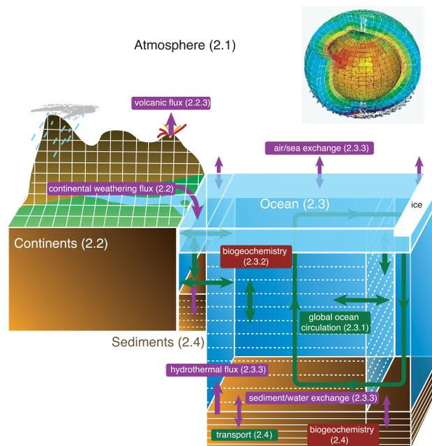
**Fig. 1.** General structure of GEOCLIM *reloaded*. A detailed description of transport (green) and transformation (red) processes within each compartment, as well as of the exchange fluxes through their interfaces (purple) is given in the sections indicated in brackets.
