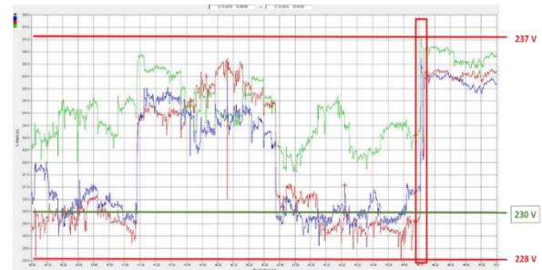
Figure 11 – Voltage measurement during islanding
