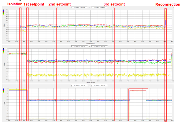
Figure 13 - LV network isolation test
