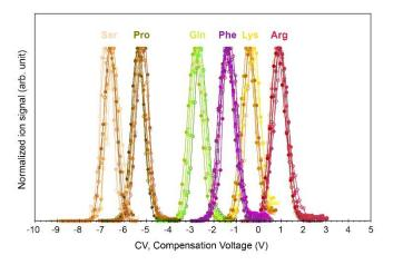
**Fig. 4** Selected DMS spectra recorded for serine (Ser), proline (Pro), glutamine (Gln), phenylalanine (Phe), lysine (Lys) and arginine (Arg) over a period of 6 months. Experiments were performed with plasma samples (filled circles) and standards of AAs and related compounds in water:methanol solutions (open circles). The mean CV and associated standard deviation values are given in Table 1. A CV value of 1 V corresponds to an electric field of 1.43 kV.m<sup>-1</sup> or ~0.07 Td.
