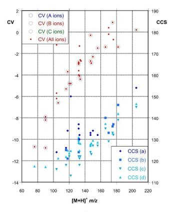
**Fig. 2** CV and CCS as a function of m/z for a selected set of AAs and related species (See list in Table S4). CV values (in V), 1 V corresponding to an electric field of 1.43 kV.m<sup>-1</sup> or  $\sim$ 0.07 Td. CCS (in Å<sup>2</sup>) are taken from (a) ref. 36, (b) ref. 31, (c) ref. 17, and (d) ref. 49.
