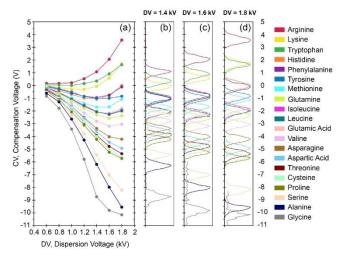
**Fig. 1** Differential ion mobility data for the 20 protonated AAs recorded at different dispersion voltage (DV) using  $N_2$  as carrier gas. (a) DMS dispersion plots, or evolution of CV as a function of DV; DMS spectra for each individual AA at DV = 1.4, 1.6, 1.8 kV are given in panels (b), (c), and (d), respectively. A CV value of 1 V corresponds to an electric field of 1.43 kV.m<sup>-1</sup> or ~0.07 Td. To facilitate visualization, each DMS peak is individually normalized.
