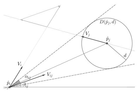
Figure 2: Geometrical analysis of conflict between two aircraft based on relative velocity
