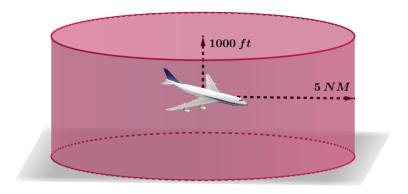
Figure 1: Safety cylinder around aircraft
