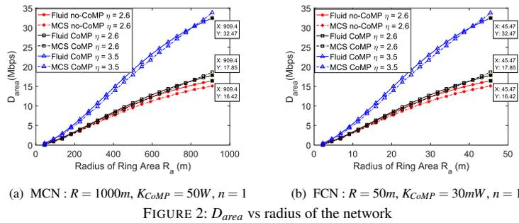
FIGURE 2:  $D_{area}$  vs radius of the network
