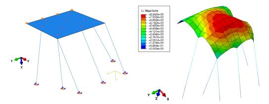
Figure 13: Geometry, boundary conditions and total displacement of the structural multicomponent model subjected to hydrostatic pressure, comprised of an anisotropic hyperelastic plane shell section which is non-symmetrically supported by a set of hyperelastic truss elements.
