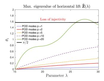
Figure 16: Stability (C2); Computation of the maximum eigenvalue  $\theta_1$  of the horizontal lift  $\tilde{\mathbf{Z}}(\lambda)$  over the parametric range [15; 30]. Observe the loss of injectivity in a specific interval of parameters for POD modes p=20. Reference point on Grassmann manifold  $\mathbf{m}_0(\lambda=15)$ .
