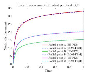
Figure 12: POD ROM-FEM model using Lagrange interpolation; comparison of the displacement of radial points A,B and C against the high-fidelity FEM solution; training points:  $\mathbf{m}_0(\lambda = 85)$  (reference point);  $\mathbf{m}_1(\lambda = 50)$ ;  $\mathbf{m}_2(\lambda = 60)$ ;  $\mathbf{m}_3(\lambda = 90)$ ; target point:  $\tilde{\mathbf{m}}(\lambda = 75)$ ; POD modes p = 1.
