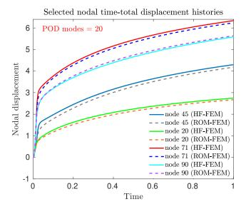
Figure 20: POD ROM-FEM; comparison of selected nodal time-displacement histories against the high-fidelity FEM solution; training points:  $\mathbf{m}_0(\lambda = 15)$ ;  $\mathbf{m}_1(\lambda = 20)$ ;  $\mathbf{m}_2(\lambda = 25)$ ;  $\mathbf{m}_3(\lambda = 30)$ ; target point:  $\tilde{\mathbf{m}}(\lambda = 17.5)$ ; POD modes = 20.
