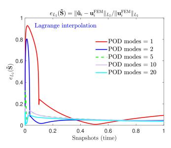
Figure 17: POD ROM-FEM; relative  $L_2$ -error norm  $e_{L_2}(\tilde{\mathbf{S}})$  against the number of POD vectors; target point:  $\tilde{\mathbf{m}}(\lambda = 17.5)$ .
