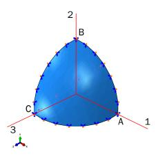
Figure 2: Geometry of an octant  $S_0$  of a spherical balloon made of transversely isotropic hyperelastic material. Three radial points A, B and C are defined on axis 1,2 and 3, respectively; plane symmetry boundary conditions are used.
