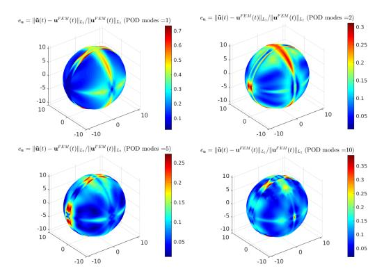
Figure 10: Relative displacement error  $e_{\mathbf{u}} = \|\tilde{\mathbf{u}}(t) - \mathbf{u}^{FEM}(t)\|_{L_2} / \|\mathbf{u}^{FEM}(t)\|_{L_2}$  at the nodal points at state t = 0.002 for POD modes  $p = \{1, 2, 5, 10\}$  displayed at the position vector  $\mathbf{x}^{FEM}(t)$  of the high-fidelity FEM model; target point:  $\tilde{\mathbf{m}}(\lambda = 75)$ .
