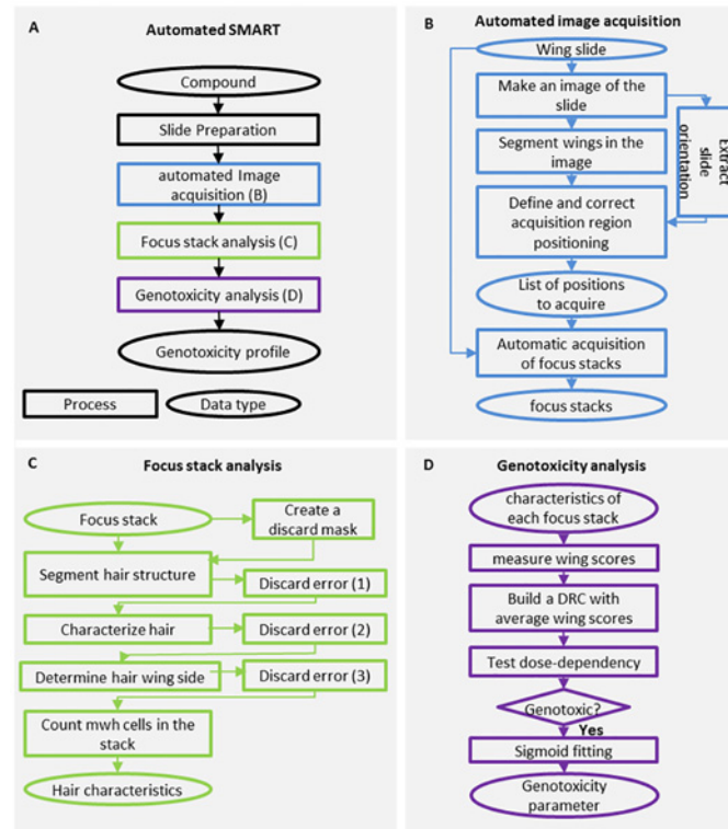
Fig 2. Automated SMART process. The methods used to automate the SMART are depicted with a flow diagram. The general flow of the method is described in (A). Each step in the process is depicted by a rectangle, with data inputs and outputs depicted using elliptical shapes. (B) Steps in automated acquisition. (C) Steps in focus stack analysis and the extraction of data on mwh hairs, cells, and spots. Discard error (1–3) refers to detection of (1) abnormal hair shape, (2) abnormal hair orientation, and/or (3) abnormal position relative to the wing surface. (D) Steps in the construction of the genotoxicity wing score dose-response curve and the characterization of compound genotoxicity.
