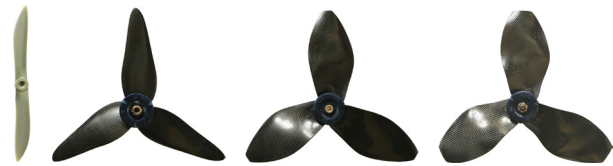
Figure 37. Tested rotors. From left to right: APC, BEMT opt. (100 g), FVM opt. (100 g), FVM opt. (300 g)
