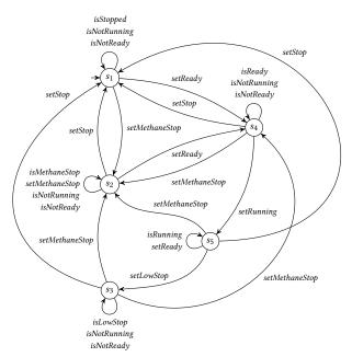
Figure 8: The state FTS of the mine pump model from [27]
