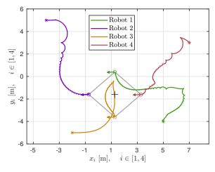
Fig. 2. Trajectories and formation of the network of mobile robots.
