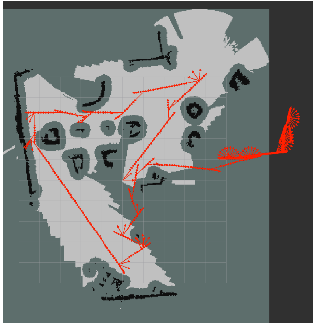
Figure 13: Costmap and robot trajectory during the contest.
