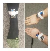
Figure 5: Haptic bracelets secured to the student's wrists and right ankle.
