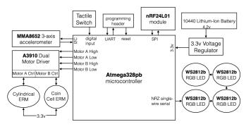
Figure 2: A system overview showing the hardware configuration of a single Vibropixel.
