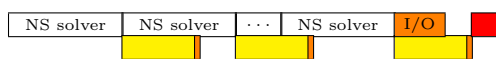
Figure 6: Revisited in situ co-processing analysis, solver on 2048 cores for 512 MPI partition, 16 cores for co-processing, 14 Go output data.
