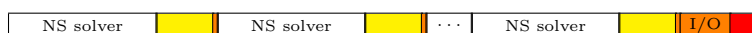
Figure 5: Tightly coupled in situ solution, when the cores for the solver are shared with the analysis.
