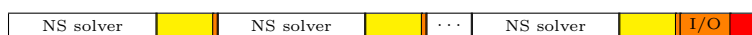
Figure 5: Tightly coupled in situ solution, when the cores for the solver are shared with the analysis.
