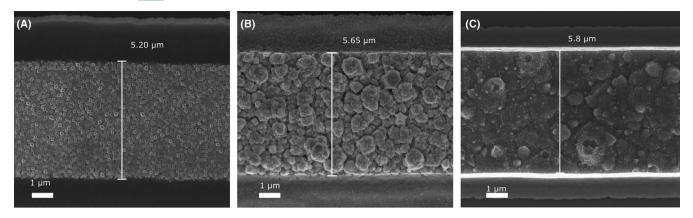
FIGURE 11 (A) Top-view SEM picture of a Ni plated line. (B) Top-view SEM picture of a Ni/Au plated line. (C) Top-view SEM picture of a Ni/Au/Ag plated line
