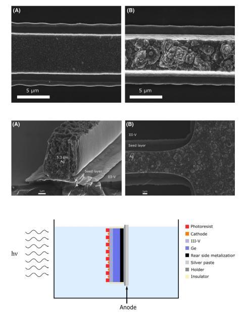
**FIGURE 7** (A) Cross-section SEM picture of a thick Ag front contact deposited by SP-LIP (4 mA/cm<sup>2</sup>) on an evaporated seed layer. (B) Top view of the same sample, at the junction between a gridline and the busbar
