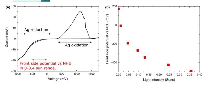
**FIGURE 3** (A) Cyclic voltammetry measurement for a noncyanide silver solution using a SCE reference electrode. (B) Front side potential measured versus the silver anode at different light intensities between 0 and 0.4 sun
