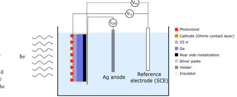
**FIGURE 2** Electrochemical characterization setup used with the silver solution.  $I_{\text{LIP}}$  is the current measured between the rear side of the cell and the Ag anode.  $V_{\text{FS}}$  is the potential of the front side and  $V_{\text{RS}}$  is the potential of the rear side. The solar cell voltage is defined as  $V_{\text{RS}}$ - $V_{\text{FS}}$
