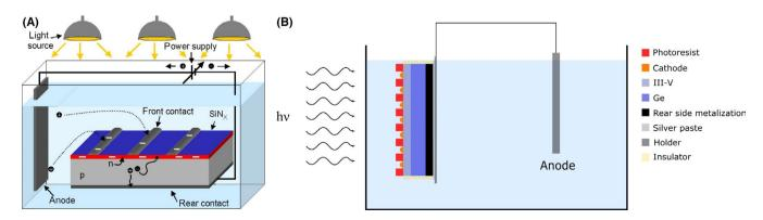
**FIGURE 1** (A) Setup for LIP deposition used by Mette et al<sup>7</sup>. (B) Setup for self-powered LIP (SP-LIP) deposition, anode is generally Ag, Ni, or Pt electrodes depending on the deposited metal
