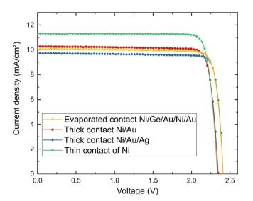
**FIGURE 10** J-V measurements under 1 sun illumination of solar cells with different emitter contacts deposited only by SP-LIP. The measurement on a solar cell with evaporated contact is set as a reference. The results presented were measured on solar cells without ARC
