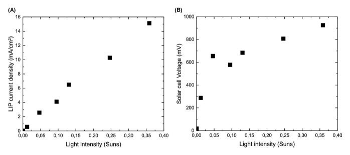
**FIGURE 4** (A) LIP current density measurements plotted against light intensity using a III-V/Ge solar cell structure. (B) Solar cell voltage  $(V_{RS}-V_{FS})$  measurements plotted against light intensity using a III-V/Ge solar cell structure
