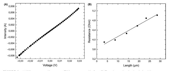
**FIGURE 9** (A) I-V curve measured between two TLM pattern separated by 5  $\mu$ m. (B) The resistance plotted against the length between two metallic patterns after a 430°C annealing. TLMs were made in a 50-nm-thick nickel layer
