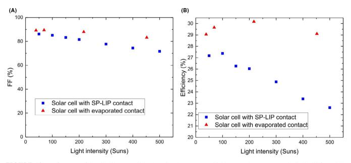
**FIGURE 12** Performances of the Ni/Au/Ag 5-µm-thick solar cell under concentrated light compared to an evaporated cell. (A) Fill factor (FF) as a function of light intensity. (B) Efficiency as a function of the light intensity
