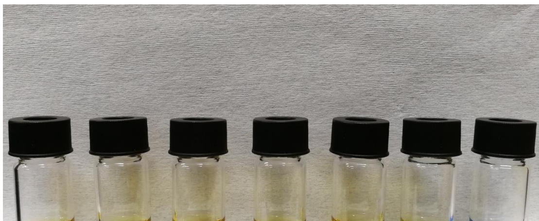
Figure S6. Image of L-Cys-MoO 2 samples with addition of 0, 200, 400, 600, 800, 1000 and 10 4 μM of H 2 O 2 .
