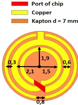
Fig. 2. Geometry of the loop antenna (units: mm).
