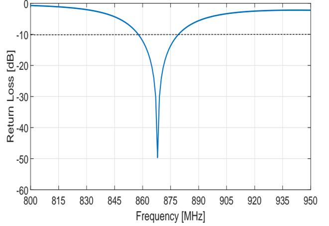
Fig. 6. Reflection coefficient of the proposed antenna.
