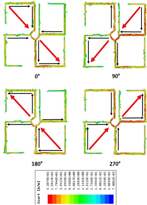
Fig. 4. Surface current distribution at 868 MHz.
