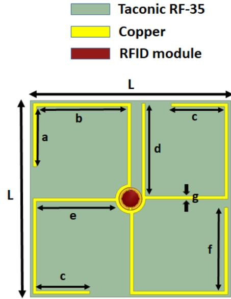
Fig. 3. Geometry of the proposed tag antennas.
