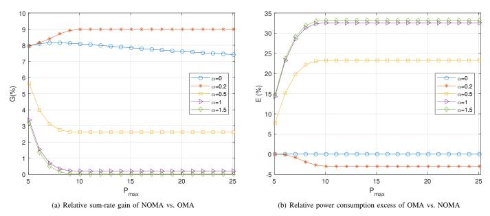
Fig. 2. NOMA vs. OMA as a function of the maximum power  $P_{\text{max}}$  for different values of  $\alpha$ . NOMA always performs at least as good as OMA in terms of sum rate and the gap between them decreases with  $\alpha$ . In terms of power consumption, for rate-driven objectives (small values of  $\alpha$ ) OMA may consume less power (down to 4%) than NOMA. At the opposite, for power-efficient objectives (large values of  $\alpha$ ) OMA consumes more power (up to 34%) than NOMA.
