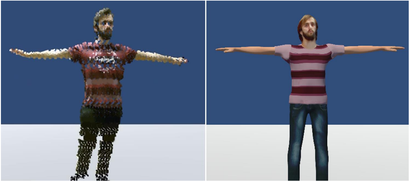
Figure 1 : Two types of the partner's representation are compared : (left) streamed point-cloud avatar and (right) preconstructed and animated virtual avatar
