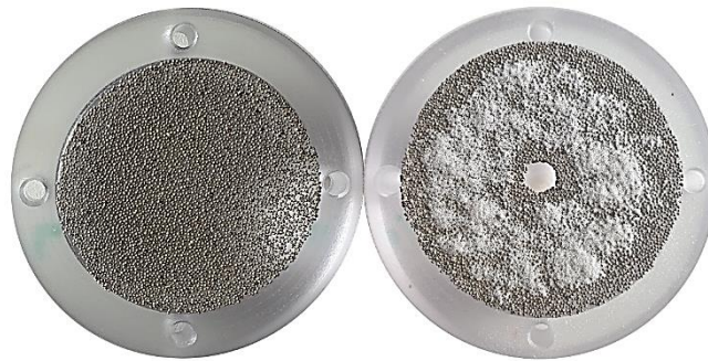
Fig. 8. Example of a fracture filled with 2 layers of proppant mesh 30/50 and clogged with 25% of natural crushed sand (Fines present in white color on the right side).
