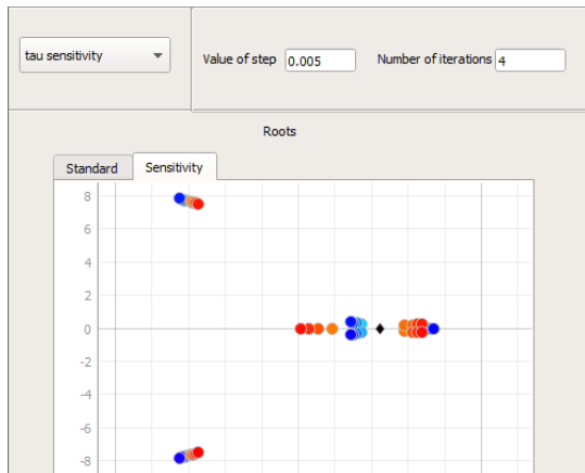
Fig. 3. Detail of the P3\delta screen for computing sensitivity with respect to the delay.
