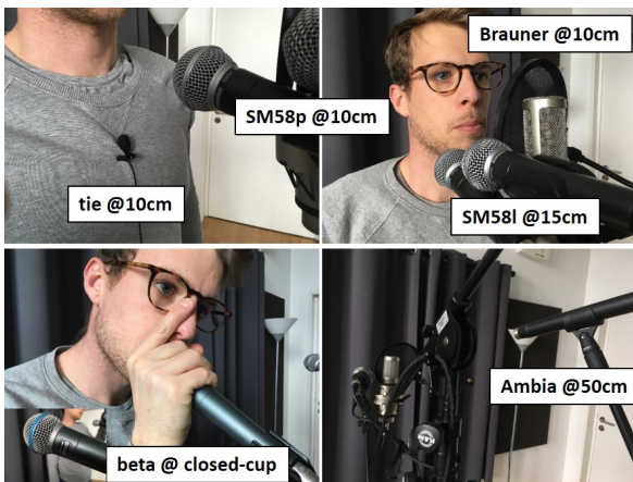
Figure 2: Placement of all microphones : tie, Braun, SM58 at 10cm and 15 cm, ambient at 50 cm, and Beta SM58 with closed-cup technique
