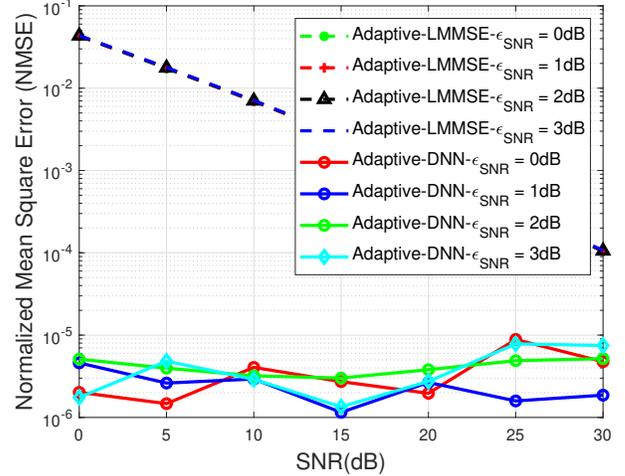
Fig. 4. NMSE Performance for Imperfect SNR Estimation.
