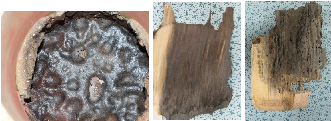
Figure 2 : (left) Photograph of Ex-vessel black in its crucible. Cut views of Ex-Vessel (center) and In-Vessel (right) fuel debris simulant synthesized at the PLINIUS platform.
