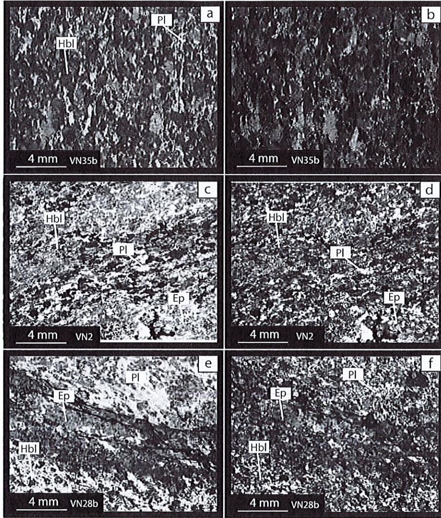
**Fig. 3.** Representative thin section microphotographs of Kef Lakhel amphibolites and metagabbros. a-b) amphibolite VN35b with hornblende porphyroblast and finely crystallized plagioclase and quartz; c-d) amphibolite VN2b with oxide-rich epidote levels; e-f) metagabbro VN28b rich in epidote, with some levels containing plagioclase, quartz and hornblende. Abbreviations are the followings: Pl: plagioclase, Ep: epidote, Hbl: hornblende.
