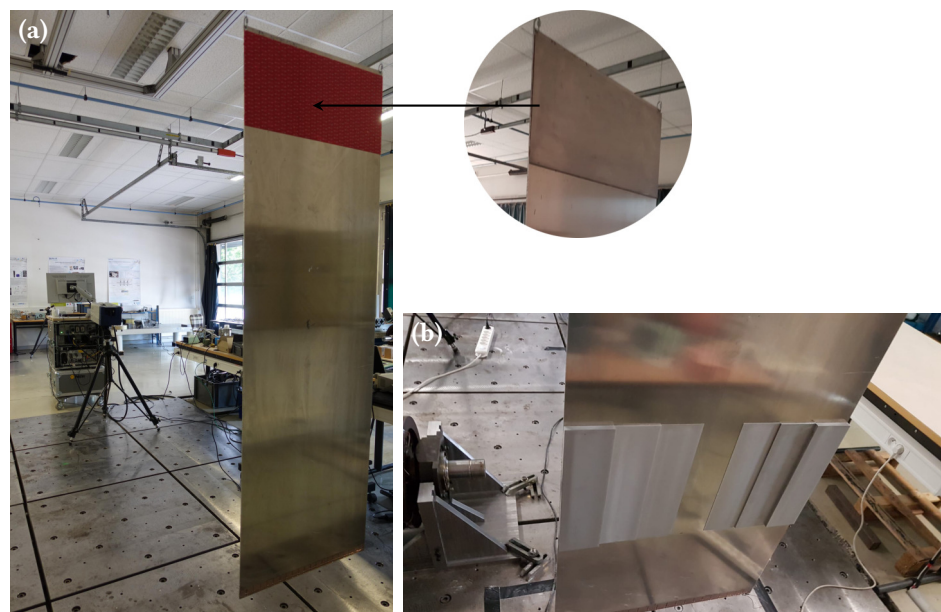
Figure 11 Experimental setup: (a) Nude plate suspended to a frame with piezoelectric patches at the lower edge and a constrained viscoelastic layer at the top edge; (b) View of the discrete GRIN lens bonded on the plate.
