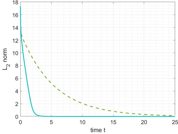
Fig. 4. Case 1: The time evolution of the spatial norm  $\mathcal{L}_2$  of  $X(t, \cdot)$  in closed-loop (solid-line) and open-loop (dashed-line)
