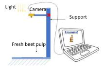
Figure 49: The device for capturing images.
