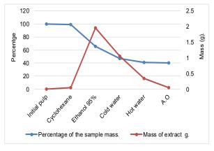
Figure 59: The percentage of the mass of fresh pulp during the various extraction stages.
