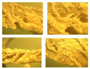
Figure 53: Microscopic photos of pulp x2.
