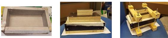
Figure 52: Photos of wooden molds used to make composite.
