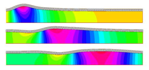
FIGURE 1. Snapshots of the fluid pressure and solid deformation at  $t = 5 \cdot 10^{-3}$ ,  $10^{-2}$  and  $1.5 \cdot 10^{-2}$  (from top to bottom). Algorithm 2 with  $\tau = 2.5 \cdot 10^{-4}$ , h = 0.05 and  $\alpha = 500$ .
