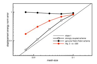
FIGURE 3. Time-convergence history of the displacement at t = 0.015, with  $\Delta t = O(h)$  obtained with Algorithm 2 ( $\alpha = 500$ ), the strongly coupled scheme and the genuine Robin-Robin explicit coupling scheme from [13, Algorithm 4].
