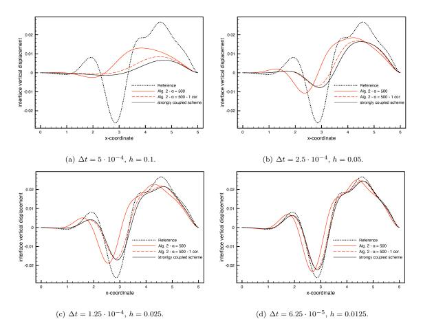
FIGURE 5. Comparison of the displacements at t = 0.015 obtained for different levels of space-time refinement,  $\Delta t = O(h)$ .
