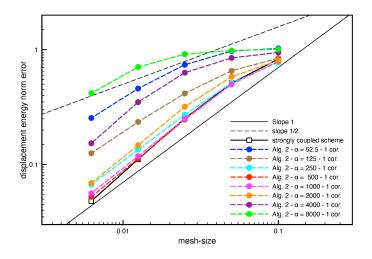
FIGURE 7. Time-convergence history of the displacement at t = 0.015, with  $\Delta t = O(h)$  obtained with Algorithm 2 with 1 correction iteration for different values of  $\alpha$ .
