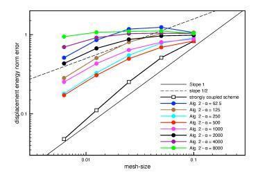
FIGURE 6. Time-convergence history of the displacement at t = 0.015, with  $\Delta t = O(h)$  obtained with Algorithm 2 for different values of  $\alpha$ .
