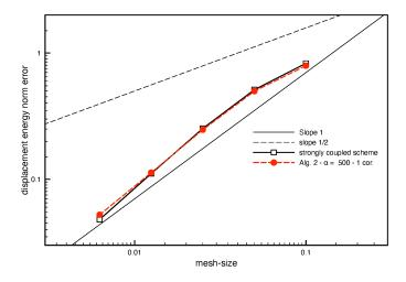
FIGURE 4. Time-convergence history of the displacement at t = 0.015, with  $\Delta t = O(h)$  obtained with the strongly coupled scheme and Algorithm 2 with 1 correction iteration ( $\alpha = 500$ ).
