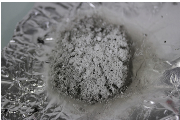
Fig. 6. Mixture of colemanite and ATH after 10 min of exposition under the epiradiator.
