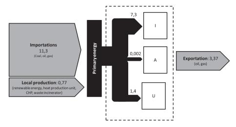
Fig. 4. Simplified energy metabolism of Aix-Marseille Provence metropolitan port area in Mtoe/year (year of reference: 2007).
