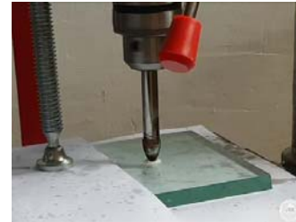
Figure 1. Glass drilling process.
