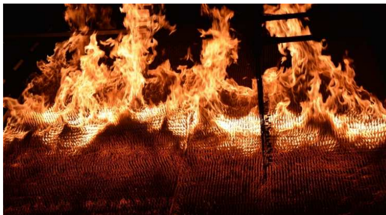
Fig. 2. Typical crest-and-trough structure of 2-m high flame observed in [16, 17] (Photo by D. Morvan at the Missoula Fire Sciences Laboratory).
