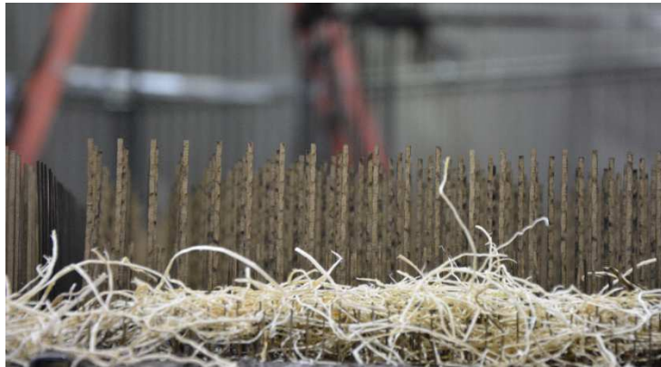
Fig. 1. Picture of the laser-cut cardboard laboratory fuel-bed used in [16, 17] (Photo by D. Morvan at the Missoula Fire Sciences Laboratory), with a line of alcohol-imbibed excelsior (in the foreground) added for the ignition of the cardboard bed.
