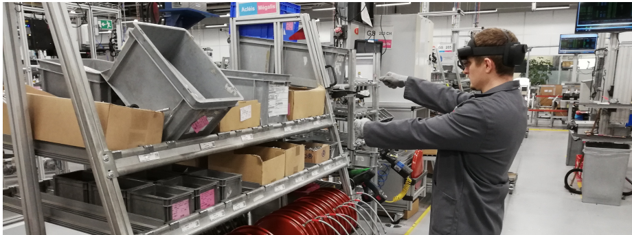
Figure 1. Operator on an assembly line using AR guidance to select components
