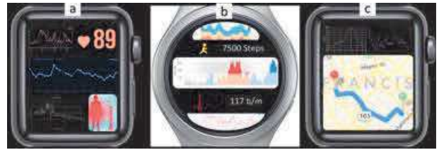
Figure 9: G-Spark applications. a) Adding more details and information, b) using G-Sparks for more complex line graphs in round faced smartwatches, and c) can be embedded in different applications, helping users with decision-making tasks.
