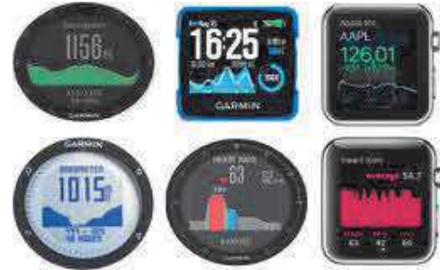
Figure 1: Line graphs are one of the most common data visualization techniques on smartwatches to represent large time-series data collected by sensors.
