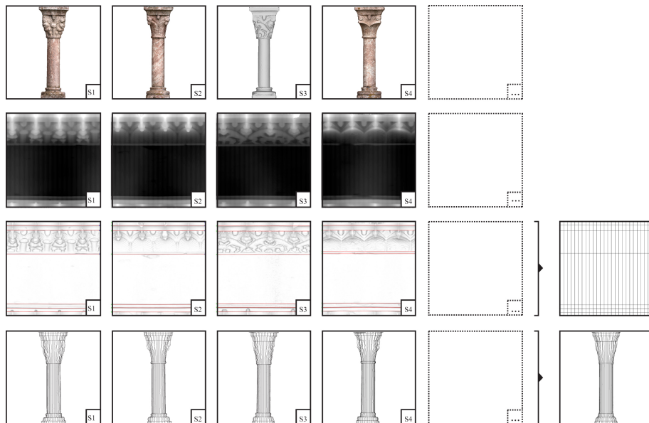
Fig. 6. A comparative analysis of four columns : from left to right, the polygonal mesh, the produced depth map, the extracted discontinuities, the created simplified geometric reconstruction and the average values.
