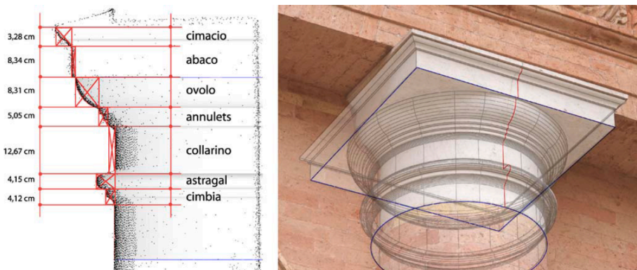
Fig.4 . Primitive adjusted on the point cloud. On the left, vertical profile with dimensional information; on the right, primitive projected on a photography oriented on the point cloud
