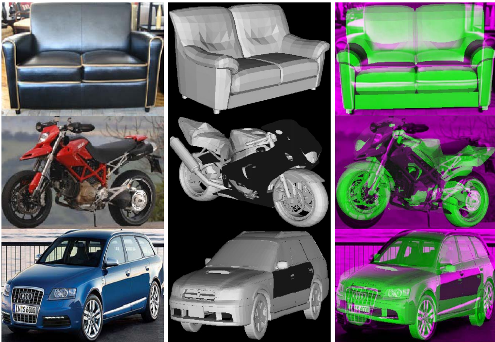
Fig. 9. Some correct registration examples with the Pascal+3D dataset. We show the query image (column 1), the corresponding 3D model (column 2) and the first ranked pose estimation (column 3). This illustrates that even if the 3D model does not have the same detailed shape, the registration can be correctly executed.
