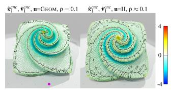
**Figure 11:** First principal curvatures and directions on polyhedral mesh "Octaflower" and its digitization.
