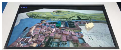
Fig. 7. Tangible table : the pose of a 3D printed object, that represents a church, highlights all the religious buildings in the virtual plan-relief
