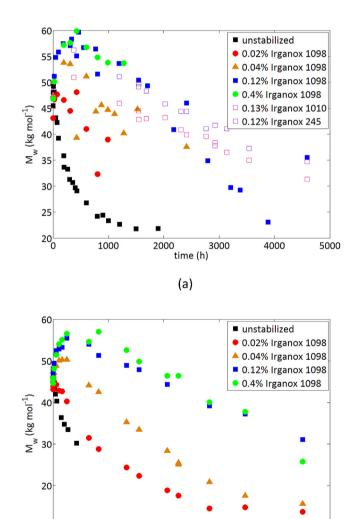
**Fig. 7.** Weight molar mass changes for unstabilized PA11 and PA11 stabilized with various levels of Irganox 1098 for exposures under air at 110  $^{\circ}$ C (a) and 90  $^{\circ}$ C (b).
