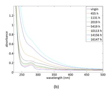
Fig. 8. UV spectra of unstabilized PA11 (a) and PA11 + 0.4% Irganox 1098 aged under air at 90  $^\circ\text{C}.$
