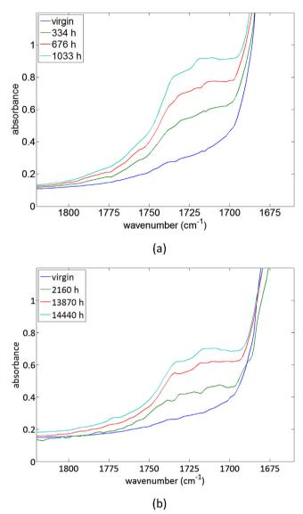
**Fig. 2.** Fourier-transform infrared spectra of unstabilized PA11 (a) and PA11 + 0.5% Irganox 1098 (b) after several ageing durations at 110 °C under atmospheric air.
