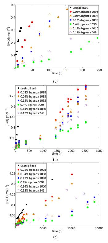
**Fig. 3.** Kinetic curves for the carbonyl build-up for unstabilized PA11 and PA11 stabilized with various levels of Irganox 1098, Irganox 1010, and Irganox 245 for exposures under air at 165 °C (a), 130 °C (b), and 90 °C (c).
