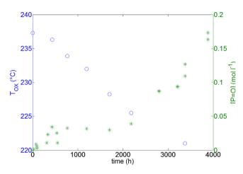
Fig. 6. Kinetic curves for carbonyl build-up and phenol depletion for PA11 + 0.12% Irganox 1098 aged at 110  $^\circ C$  under atmospheric air.
