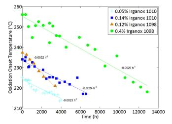
Fig. 5. Oxidation onset temperature changes for PA11 stabilized with various levels of Irganox 1098 and Irganox 1010 for exposures under air at 110  $^\circ$ C.
