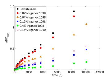
Fig. 9. Yellowing changes for unstabilized PA11 and PA11 stabilized with various levels of Irganox 1098 aged under air at 90  $^\circ$ C.
