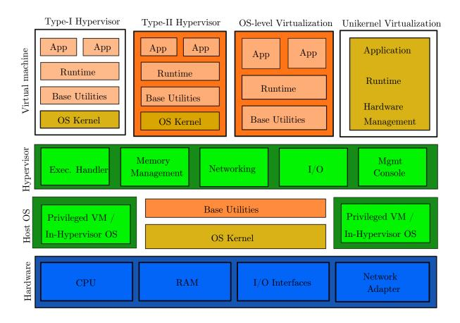
Figure 2: Virtualization reference architecture.
