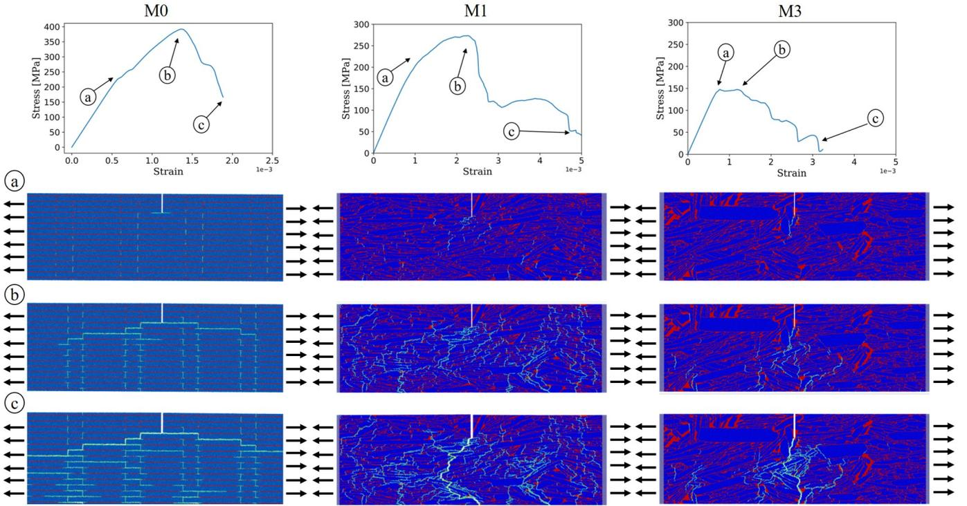
Fig. 5: Crack propagation illustrations in microstructures M0, M1 and M3 for a low interface strength ( $\Sigma_i = 1/20 \Sigma_t = 200$  MPa). Stress-strain curves and snapshots of the three main events during SENT **(a)** damage initiation, **(b)** maximum stress and **(c)** sample failure.
