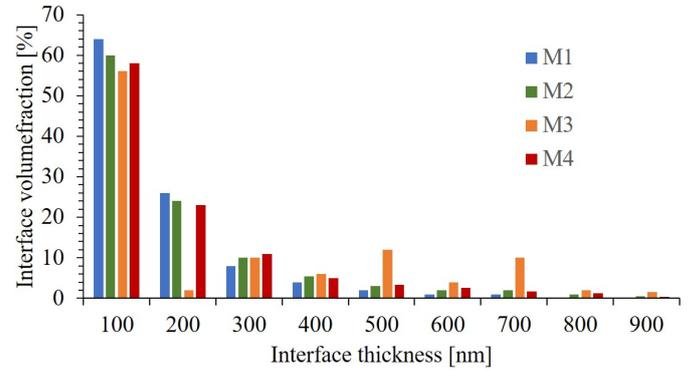
Fig. 2: Histogram of interfaces thickness for the EBSD microstructures, showing the occurrence of thicker interfaces in M3.
