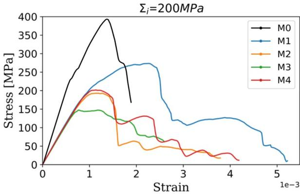
Fig. 3: An example of stress-strain curves of single edge notched samples for the five microstructures (M0-M4) with an interface strength  $\Sigma_i = \frac{1}{20}\Sigma_t = 200$  MPa and a fixed tablet strength of 4 GPa.
