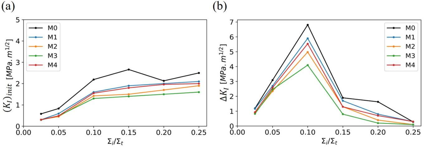
Fig. 4: a) Crack initiation stress intensity factor  $(K_I)_{init}$  and b) crack propagation toughening  $\Delta K_I$  of the regular microstructure (M0) and the EBSD generated microstructures (M1-4) as a function of the normalized interface strength  $\frac{\Sigma_i}{\Sigma_t}$ .
