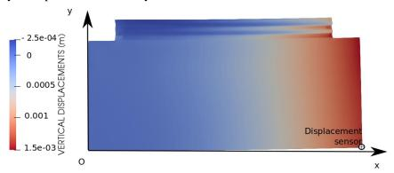
Figure 13: vertical displacement of the BP and deposits once the whole temperature dropped to the room temperature (20°C).
