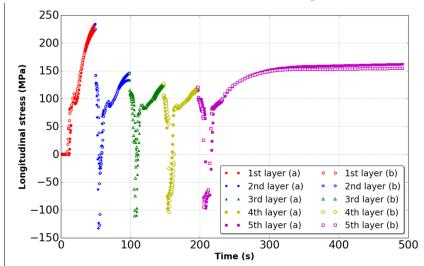
Figure 12: evolution of the longitudinal stress  $(\sigma_{xx})$  for a point in the first layer (x=80 mm and y = 51 mm as shown in figure 9) for two deposition strategies: (a) the layers are deposited alternatively that is to say that the deposit origin is the end of the previous one; (b) the layers are deposited in the same direction from the same origin.
