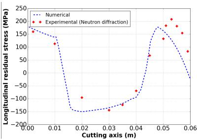
Figure 11: comparison between numerical and measured longitudinal residual stresses  $\sigma_{xx}^R$ . The longitudinal stresses were measured with neutron diffraction technique at Helmholtz Centre Berlin.
