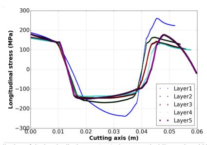
Figure 10: distribution of the longitudinal stress  $(\sigma_{xx})$  along a vertical line at the middle of base plate – deposits (see figure 9). The deposition strategy is alternative.
