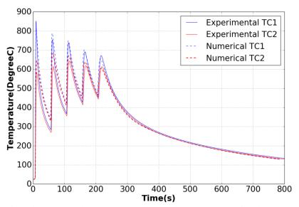
Figure 8: comparison between calculated and measured temperatures for the two sensors TC1 and TC2 located in the base plate and respectively 3 mm and 5 mm underneath the middle of the 1st deposit (see figure 7).
