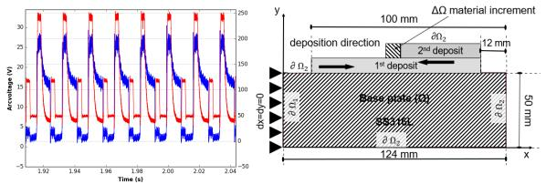
Figure 1: CMT electrical waveforms monitored during a deposition procedure (Arc Voltage is in blue and current is in red).
