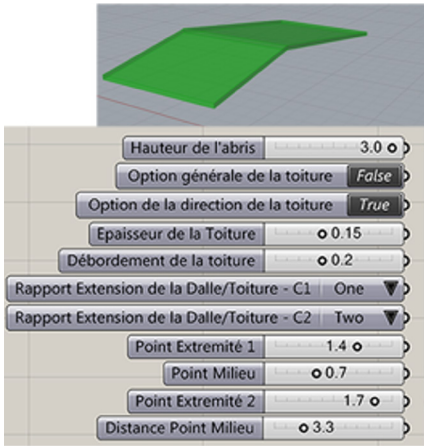
Figure 5 Roof generation process and parameters
