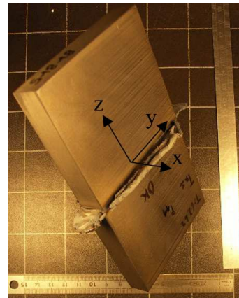
Figure 1 : a) Sketch of the geometry of the welded parts and the sampling method for observations and diffraction analysis [16] with the forging direction \langle z \rangle and the oscillating direction \langle y \rangle ; b) picture of the whole assembly. The forging part is the upper part ( z > 0 ) and the oscillating part is the lower part ( z < 0 ).
