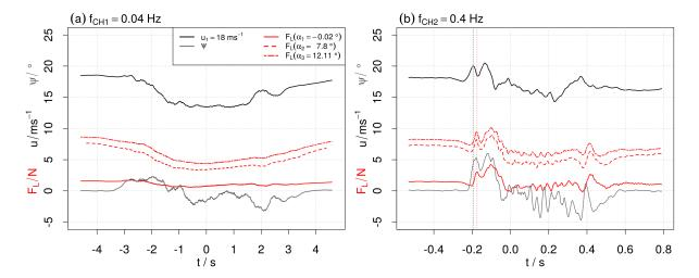
Figure 6. Airfoil's lift response to the gust: The gust velocity (black), the gust-induced flow pitch angle  $\psi$  (gray) and the lift force response for the three airfoil angles  $-0.02^{\circ}$ ,  $7.8^{\circ}$  and  $12.11^{\circ}$  (red, different line types) are plotted for  $f_{CH1} = 0.04$  Hz, (a), and  $f_{CH2} = 0.4$  Hz, (b).
