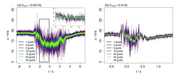
**Figure 2.** Example of one gust event (dark purple) in addition to phase averages over an increasing number of gust events to visualize the statistical convergence. The measurements were performed with a 1D hot-wire for the two chopper frequencies  $f_{CH1} = 0.04 \text{ Hz}$ , (a), and  $f_{CH2} = 0.4 \text{ Hz}$ , (b).
