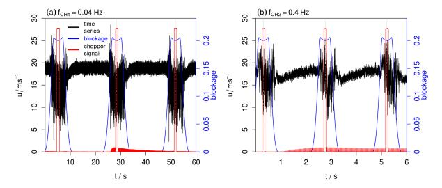
**Figure 3.** A part of the time series that shows three gusts is plotted for the two chopper frequencies  $f_{CH1} = 0.04 \,\mathrm{Hz}$ , (a), and  $f_{CH2} = 0.4 \,\mathrm{Hz}$ , (b). The measurements were carried out using a 1D hot-wire. In addition, the signal of the induction sensor is plotted in red (arbitrary units) and the blockage is plotted in blue with the corresponding blue axis at the right side of the plot.
