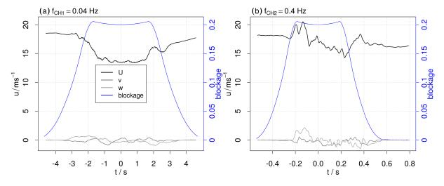
**Figure 5.** Smoothed velocity components U (black), v (dark gray) and w (light gray) for  $u_0 = 18 \,\mathrm{ms^{-1}}$  and the two chopper frequencies  $f_{CH1} = 0.04 \,\mathrm{Hz}$ , (a), and  $f_{CH2} = 0.4 \,\mathrm{Hz}$ , (b). In addition, the blockage induced by the chopper is plotted in blue.
