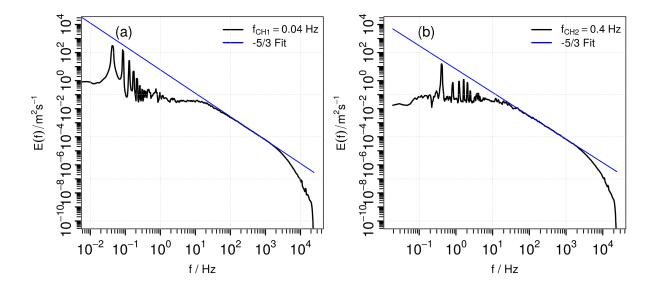
Figure 4. Energy spectral density of the stream-wise velocity component measured with a 1D hot-wire 21.5 cm in front of the airfoil ( $\alpha_{02} = 7.8^{\circ}$ ) for the two chopper frequencies  $f_{CH1} = 0.04 \text{ Hz}$ , (a), and  $f_{CH2} = 0.4 \text{ Hz}$ , (b).
