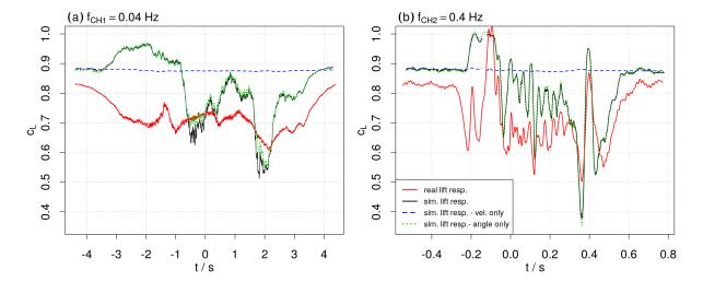
Figure 7. Simulated and calculated lift coefficient  $c_L$  at  $\alpha_{02} = 7.8^{\circ}$  for  $f_{CH1} = 0.4 \,\mathrm{Hz}$ , (a), and  $f_{CH2} = 0.04 \,\mathrm{Hz}$ , (b), respectively:  $c_L$  is simulated with respect to the gust velocity and gust-induced flow pitch angle (black), the gust-induced flow pitch angle only (green, dot-dashed), and the velocity only (blue, dashed).
