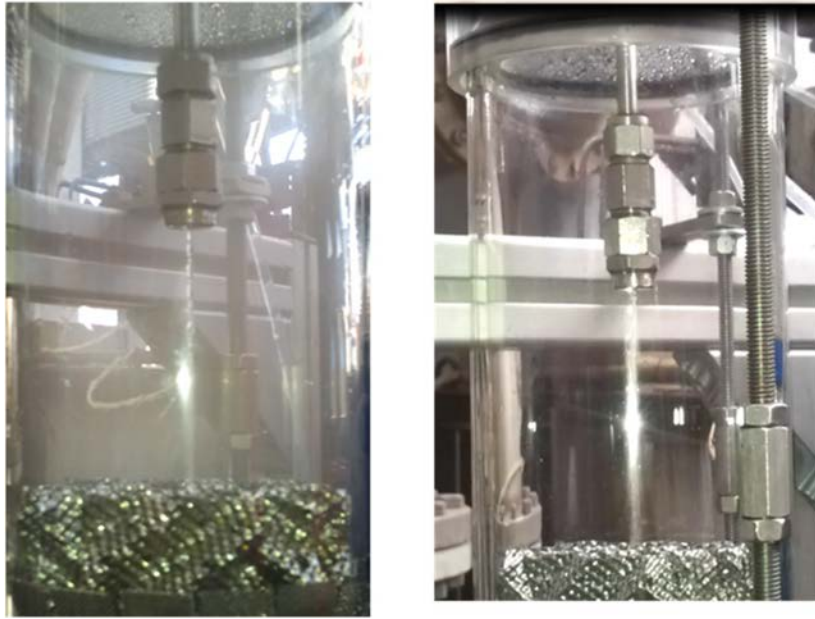
Fig. 5 Picture of the mini-absorber used at the different sampling locations (left: presence of mist formation, right: no mist formation)
